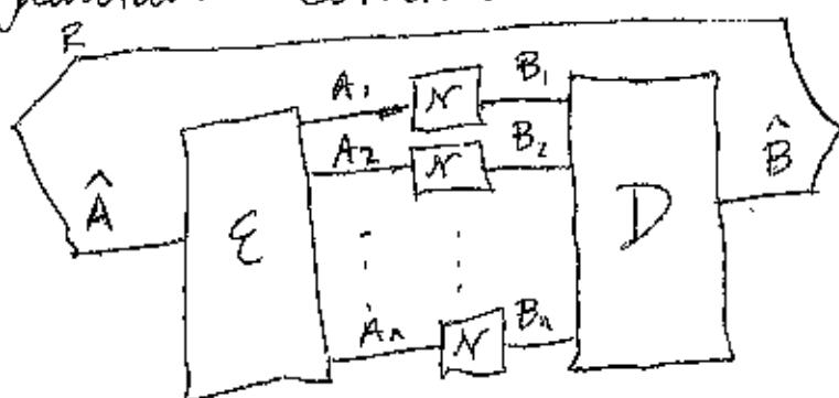
E - encoding , D - decoding
