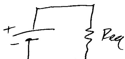
$$R_{eq} = R_1 + R_2 + R_3$$
