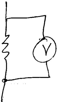
important that resistance of voltmeter be much larger than that of resistor.
