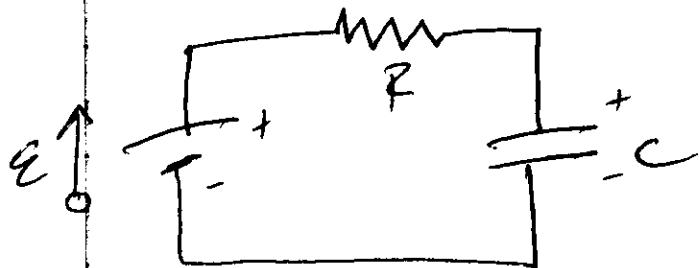
We know that when we connect the circuit, the capacitor charges up to a point where it is fully charged, & then current no longer flows.
