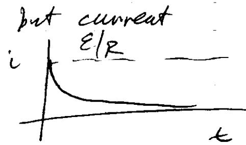
$$\begin{aligned}\frac{dq(t)}{dt} &= CE \exp\{-t/RC\} \frac{1}{RC} \\ &= \frac{E}{R} \exp\{-t/RC\}\end{aligned}$$
