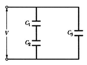
a) [7 points] Find the equivalent capacitance of the combination
